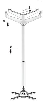
Tighten the nut (f) with a 17mm wrench.
